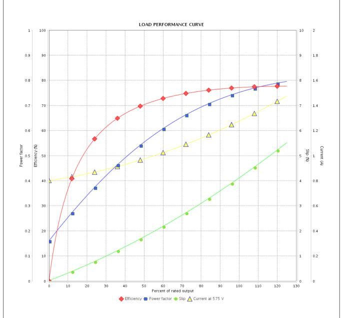
Performance : 575 V 60 Hz 2P : 1.30 A : 0.0010 kgm<sup>2</sup> Rated current Moment of inertia (J) **LRC** : 8.3 Duty cycle : Cont.(S1) : 0.210 kgfm Insulation class Rated torque : F Locked rotor torque : 400 % Service factor : 1.40 Breakdown torque : 409 % Temperature rise : 80 K Rated speed : 3450 rpm
