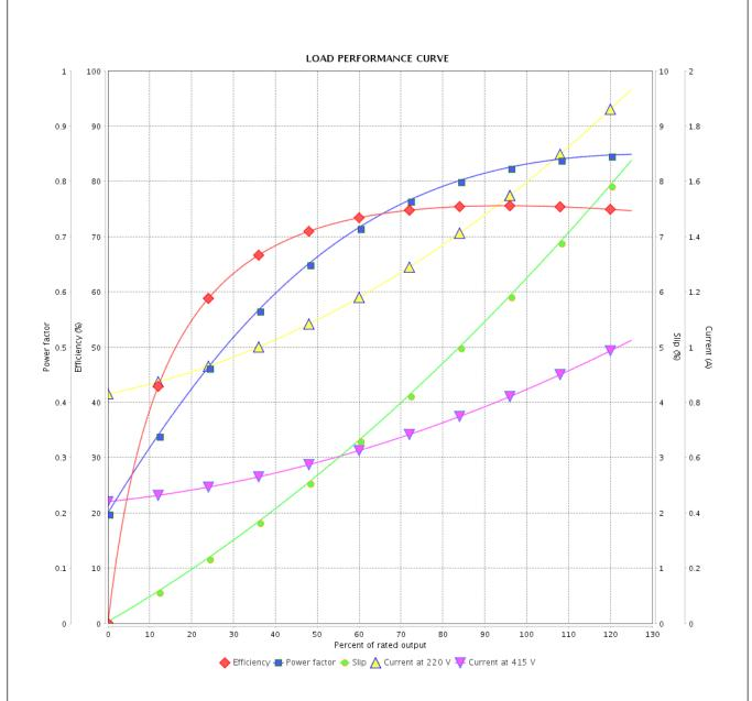
Performance : 220/415 V 50 Hz 2P : 1.61/0.852 A : 0.0008 kgm<sup>2</sup> Rated current Moment of inertia (J) **LRC** Duty cycle : Cont.(S1) : 6.4 : 0.129 kgfm Insulation class : F Rated torque Locked rotor torque : 280 % Service factor : 1.15 Breakdown torque : 280 % Temperature rise : 80 K Rated speed : 2810 rpm
