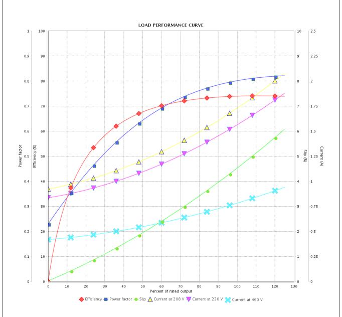
Performance : 208-230/460 V 60 Hz 2P : 1.73-1.57/0.784 A : 0.0008 kgm<sup>2</sup> Rated current Moment of inertia (J) **LRC** Duty cycle : Cont.(S1) : 7.7 : 0.106 kgfm Insulation class Rated torque : F Locked rotor torque : 330 % Service factor Breakdown torque : 360 % Temperature rise : 80 K Rated speed : 3435 rpm
