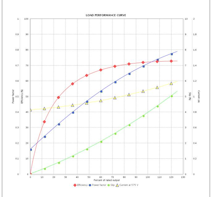
Performance : 575 V 60 Hz 2P : 1.08 A : 0.0007 kgm<sup>2</sup> Rated current Moment of inertia (J) **LRC** : 6.7 : Cont.(S1) Duty cycle : 0.158 kgfm Insulation class : F Rated torque Locked rotor torque : 330 % Service factor : 1.15 Breakdown torque : 350 % Temperature rise : 80 K Rated speed : 3455 rpm
