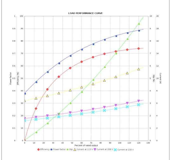
Performance : 115/208-230 V 60 Hz 4P : 10.7/5.50-5.33 A : 0.0055 kgm<sup>2</sup> Rated current Moment of inertia (J) **LRC** : 8.4 Duty cycle : Cont.(S1) : 0.436 kgfm Insulation class Rated torque : F Locked rotor torque : 270 % Service factor
