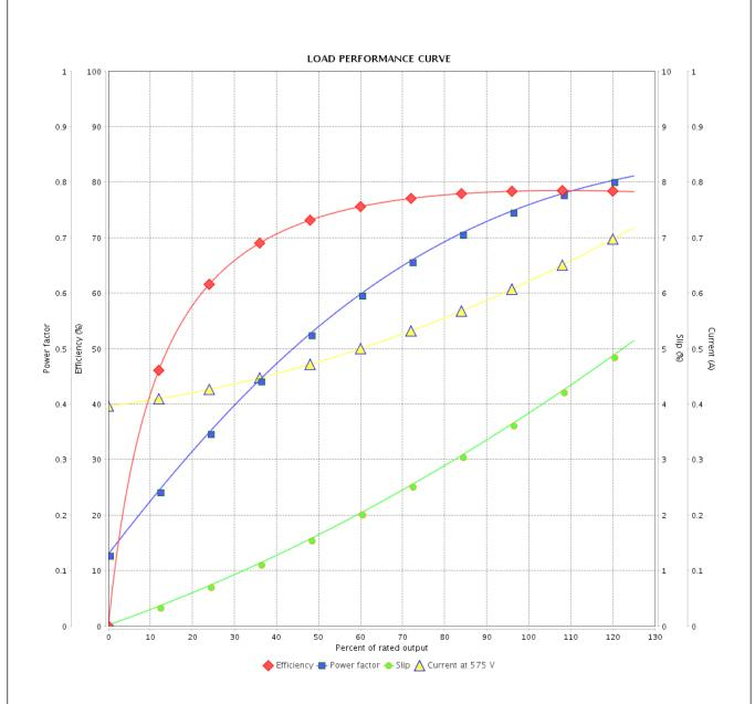
Performance : 575 V 60 Hz 4P : 0.0022 kgm<sup>2</sup> Rated current : 0.622 A Moment of inertia (J) **LRC** Duty cycle : Cont.(S1) : 6.4 : 0.210 kgfm Insulation class : F Rated torque Locked rotor torque : 229 % Service factor : 1.15 Breakdown torque : 310 % Temperature rise : 80 K Rated speed : 1730 rpm
