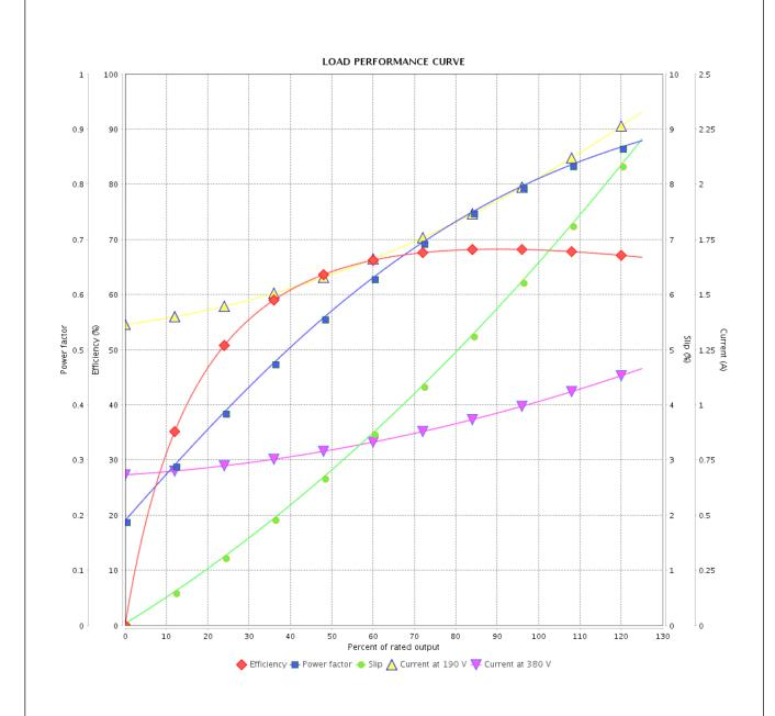
Performance : 190/380 V 50 Hz 4P Rated current : 2.04/1.02 A Moment of inertia (J) : 0.0017 kgm<sup>2</sup> **LRC** : 4.7 Duty cycle : Cont.(S1) : 0.259 kgfm Insulation class : F Rated torque Locked rotor torque : 190 % Service factor : 1.00 Breakdown torque : 200 % Temperature rise : 80 K Rated speed : 1400 rpm
