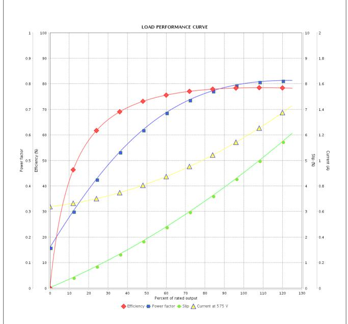
Performance : 575 V 60 Hz 2P : 1.20 A : 0.0011 kgm<sup>2</sup> Rated current Moment of inertia (J) **LRC** : 8.8 Duty cycle : Cont.(S1) : 0.211 kgfm Insulation class Rated torque : F Locked rotor torque : 360 % Service factor : 1.15 Breakdown torque : 380 % Temperature rise : 80 K Rated speed : 3435 rpm
