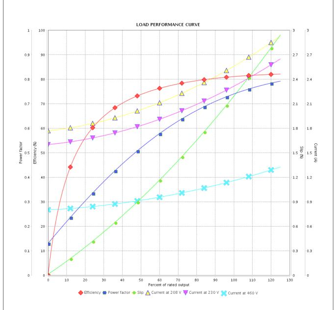
Performance : 208-230/460 V 60 Hz 4P : 2.54-2.30/1.15 A : 0.0030 kgm<sup>2</sup> Rated current Moment of inertia (J) **LRC** : 7.3 Duty cycle : Cont.(S1)
