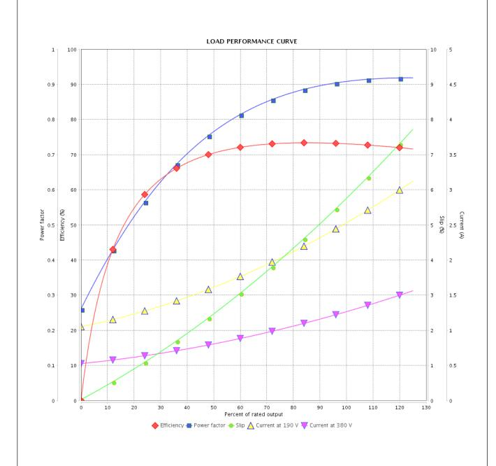
Performance : 190/380 V 50 Hz 2P : 2.52/1.26 A Rated current Moment of inertia (J) : 0.0022 kgm<sup>2</sup> **LRC** : 5.5 Duty cycle : Cont.(S1) : 0.193 kgfm Insulation class : F Rated torque Locked rotor torque : 180 % Service factor : 1.00 Breakdown torque : 220 % Temperature rise : 105 K Rated speed : 2825 rpm
