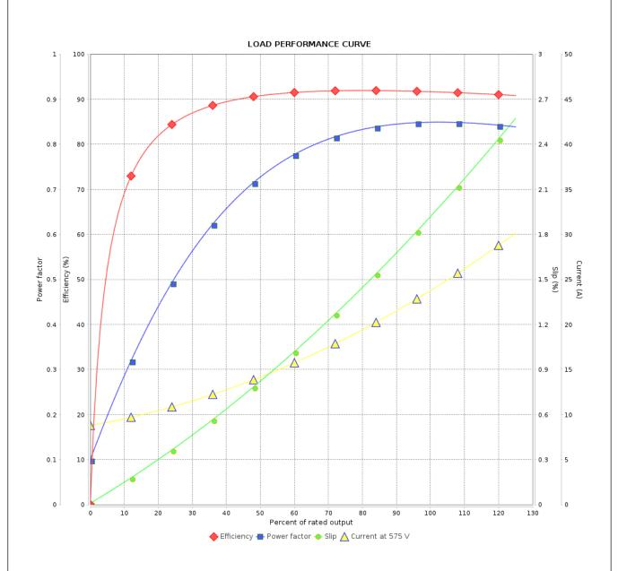
Performance : 575 V 60 Hz 2P : 0.0456 kgm<sup>2</sup> Rated current : 23.8 A Moment of inertia (J) **LRC** Duty cycle : Cont.(S1) : 6.5 Insulation class Rated torque : 5.14 kgfm : F Locked rotor torque : 200 % Service factor : 1.15 Breakdown torque : 260 % Temperature rise : 80 K Rated speed : 3530 rpm Design : B Rev. Performed Checked Date **Changes Summary** Performed by Checked by Revision Page
