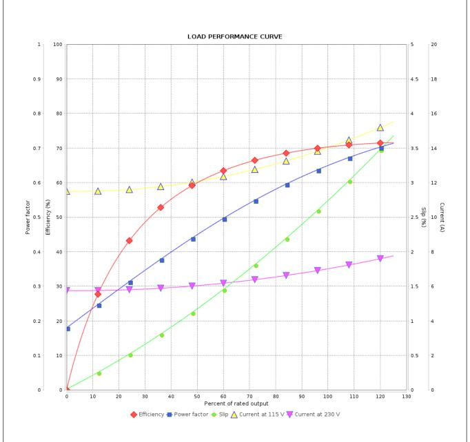
Performance : 115/230 V 60 Hz 4P : 14.0/7.00 A : 0.0056 kgm<sup>2</sup> Rated current Moment of inertia (J) **LRC** Duty cycle : Cont.(S1) : 6.5 : 0.415 kgfm Insulation class Rated torque : B Locked rotor torque : 320 % Service factor : 1.15 Breakdown torque : 270 % Temperature rise : 80 K Rated speed : 1750 rpm
