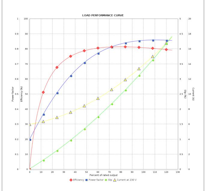
Performance : 230 V 60 Hz 4P : 14.5 A : 0.0100 kgm<sup>2</sup> Rated current Moment of inertia (J) **LRC** : 6.0 Duty cycle : Cont.(S1) : 1.25 kgfm Insulation class Rated torque : F Locked rotor torque : 260 % Service factor : 1.15 Breakdown torque : 220 % Temperature rise : 80 K Rated speed : 1740 rpm
