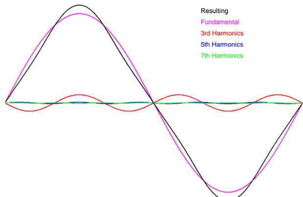
Figure 6: Harmonics with 5/6 pitch winding
