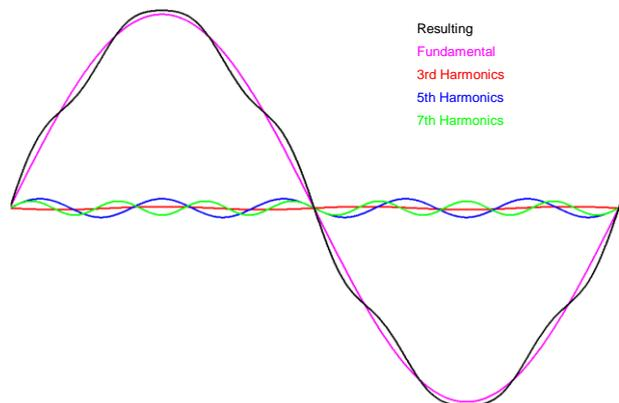
Figure 5: Harmonics with 2/3 pitch winding
