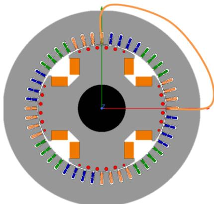
Figure 2: Full pitch winding
