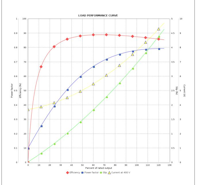
: 400 V 50 Hz 6P IE3 Performance : 7.82 A : 0.0620 kgm<sup>2</sup> Rated current Moment of inertia (J) **LRC** Duty cycle : Cont.(S1) : 6.1 Insulation class : F Rated torque : 3.76 kgfm Locked rotor torque : 160 % Service factor : 1.00 Breakdown torque : 229 % Temperature rise : 80 K Rated speed : 965 rpm Design : B Rev. Changes Summary Checked Performed Date
