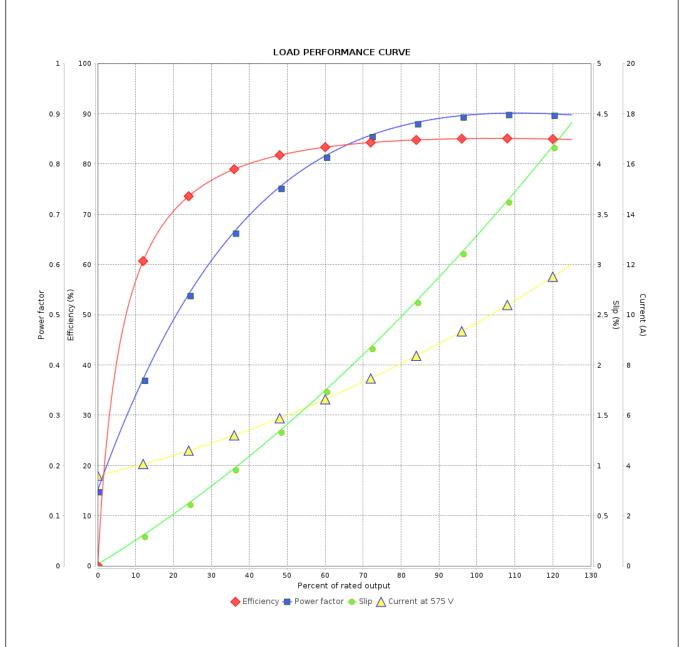
Performance : 575 V 60 Hz 2P Rated current : 9.83 A Moment of inertia (J) : 0.0140 kgm<sup>2</sup> **LRC** : 8.7 Duty cycle : S6 : 2.09 kgfm Insulation class : F Rated torque Locked rotor torque : 400 % Service factor : 1.15 Breakdown torque : 420 % Temperature rise : 80 K Rated speed : 3480 rpm Design : N Rev. Performed Checked Date **Changes Summary**
