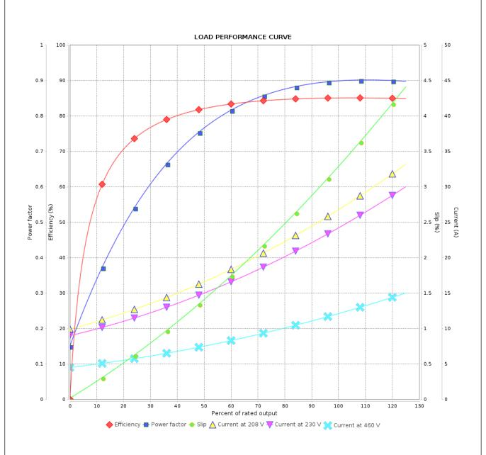
Performance : 208-230/460 V 60 Hz 2P Rated current : 27.2-24.6/12.3 A Moment of inertia (J) : 0.0140 kgm<sup>2</sup> **LRC** Duty cycle : 8.7 : S6 : 2.09 kgfm Insulation class : F Rated torque Locked rotor torque : 400 % Service factor : 1.15 Breakdown torque : 420 % Temperature rise : 80 K Rated speed : 3480 rpm Design : N Rev. Performed Checked Date **Changes Summary** Performed by Checked by Revision Page
