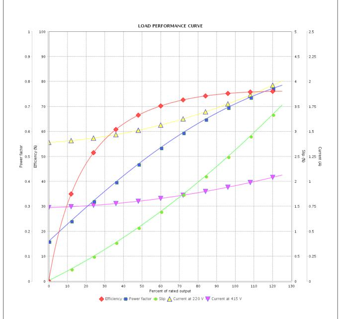
Performance : 220/415 V 50 Hz 4P : 1.81/0.962 A : 0.0025 kgm<sup>2</sup> Rated current Moment of inertia (J) **LRC** Duty cycle : Cont.(S1) : 6.3 : 0.249 kgfm Insulation class Rated torque : F Locked rotor torque : 220 % Service factor : 1.15 Breakdown torque : 310 % Temperature rise : 80 K Rated speed : 1460 rpm
