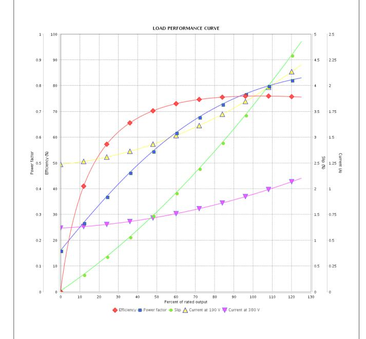
Performance : 190/380 V 50 Hz 4P : 1.90/0.950 A Rated current Moment of inertia (J) : 0.0025 kgm<sup>2</sup> **LRC** : 5.8 Duty cycle : Cont.(S1) : 0.251 kgfm Insulation class : F Rated torque Locked rotor torque : 180 % Service factor : 1.15 Breakdown torque : 250 % Temperature rise : 80 K Rated speed : 1445 rpm
