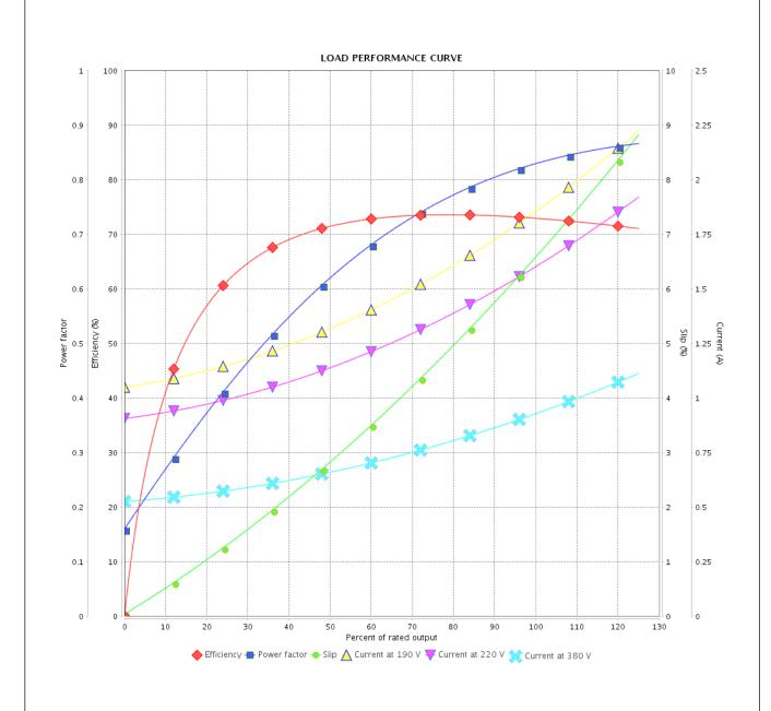
Performance : 190-220/380 V 50 Hz 4P : 1.86-1.60/0.928 A Rated current Moment of inertia (J) : 0.0019 kgm<sup>2</sup> **LRC** : 4.8 Duty cycle : Cont.(S1) : 0.259 kgfm Insulation class : F Rated torque Locked rotor torque : 180 % Service factor : 1.15 Breakdown torque : 210 % Temperature rise : 80 K Rated speed : 1400 rpm
