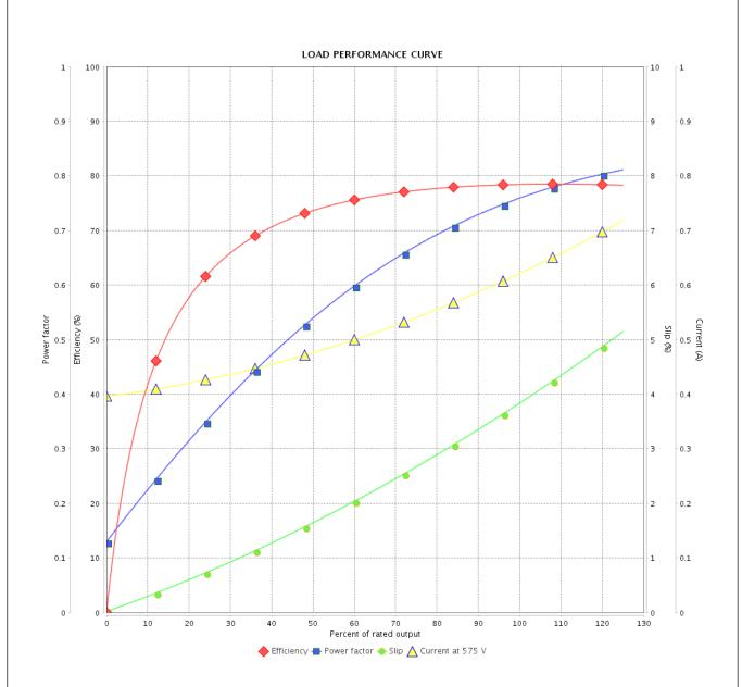
Performance : 575 V 60 Hz 4P : 0.0022 kgm<sup>2</sup> Rated current : 0.622 A Moment of inertia (J) **LRC** : 6.4 Duty cycle : Cont.(S1) : 0.210 kgfm Insulation class : F Rated torque Locked rotor torque : 229 % Service factor : 1.15 Breakdown torque : 310 % Temperature rise : 80 K Rated speed : 1730 rpm
