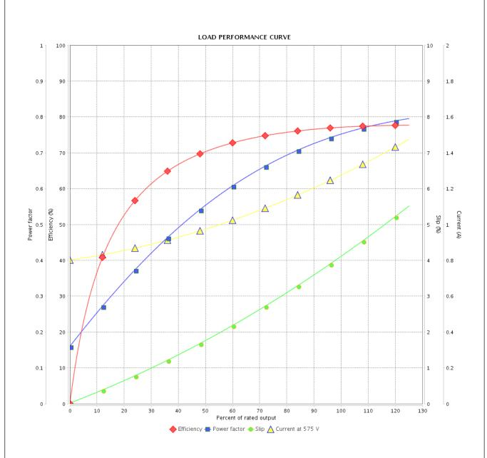
Performance : 575 V 60 Hz 2P : 1.30 A : 0.0010 kgm<sup>2</sup> Rated current Moment of inertia (J) **LRC** Duty cycle : Cont.(S1) : 8.3 : 0.210 kgfm Insulation class : F Rated torque Locked rotor torque : 400 % Service factor : 1.40 Breakdown torque : 409 % Temperature rise : 80 K Rated speed : 3450 rpm
