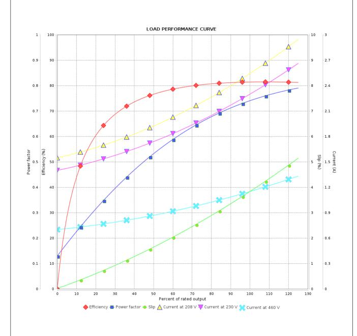
Performance : 208-230/460 V 60 Hz 4P : 2.57-2.32/1.16 A Rated current Moment of inertia (J) : 0.0041 kgm<sup>2</sup> **LRC** : 5.7 Duty cycle : Cont.(S1) : 0.315 kgfm Rated torque Insulation class : B Locked rotor torque : 240 % Service factor Breakdown torque : 280 % Temperature rise : 80 K Rated speed : 1730 rpm
