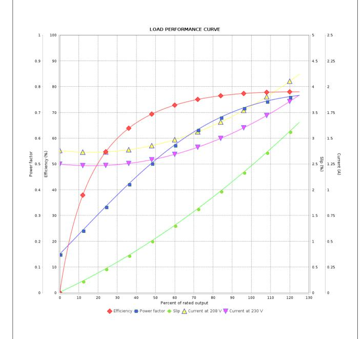
Performance : 208-230 V 60 Hz 4P : 1.80-1.63 A Rated current Moment of inertia (J) : 0.0034 kgm<sup>2</sup> **LRC** : 6.8 Duty cycle : Cont.(S1) : 0.207 kgfm Rated torque Insulation class : B Locked rotor torque : 220 % Service factor Breakdown torque : 330 % Temperature rise : 80 K Rated speed : 1755 rpm
