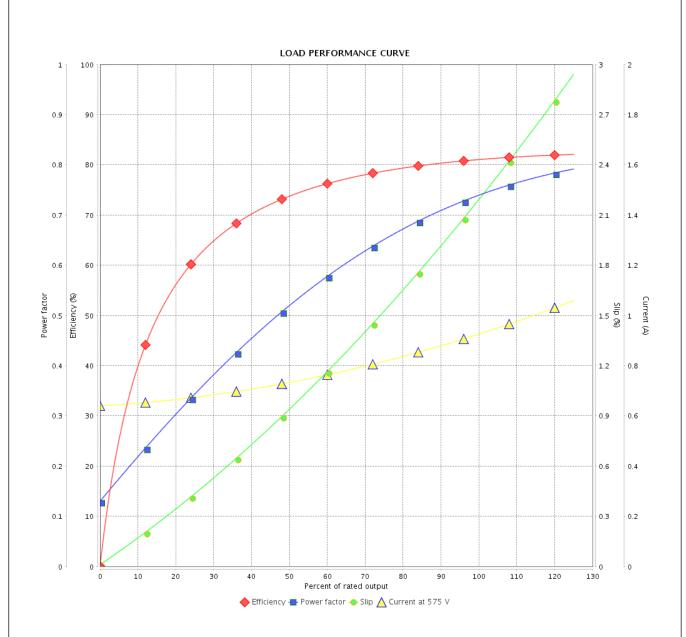
: 575 V 60 Hz 4P Performance : 0.0030 kgm<sup>2</sup> Rated current : 0.920 A Moment of inertia (J) **LRC** : 7.3 Duty cycle : Cont.(S1) : 0.309 kgfm Insulation class : F Rated torque Locked rotor torque : 250 % Service factor : 1.25 Breakdown torque : 300 % Temperature rise : 80 K Rated speed : 1760 rpm
