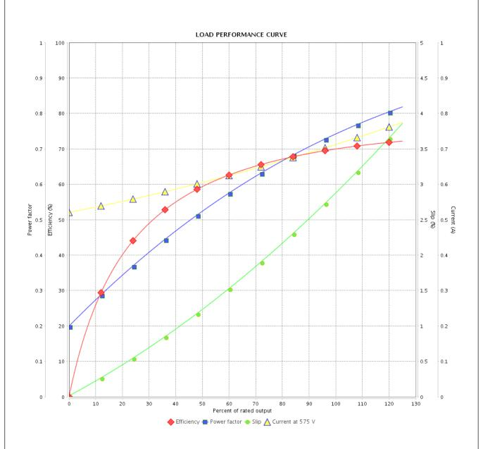
Performance : 575 V 60 Hz 2P : 0.0016 kgm<sup>2</sup> Rated current : 0.718 A Moment of inertia (J) **LRC** Duty cycle : Cont.(S1) : 6.2 : 0.104 kgfm Insulation class : F Rated torque Locked rotor torque : 229 % Service factor : 1.60 Breakdown torque : 290 % Temperature rise : 80 K Rated speed : 3495 rpm
