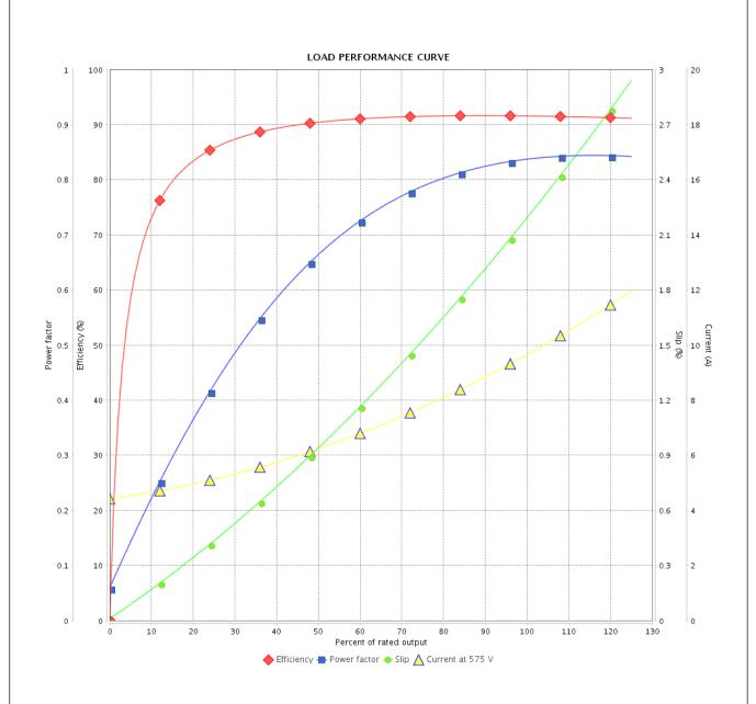
Performance : 575 V 60 Hz 4P : 0.0451 kgm<sup>2</sup> Rated current : 9.76 A Moment of inertia (J) **LRC** : 7.0 Duty cycle : Cont.(S1) : 4.12 kgfm Insulation class Rated torque : F Locked rotor torque : 250 % Service factor : 1.15 Breakdown torque : 300 % Temperature rise : 80 K Rated speed : 1760 rpm Design : B Rev. Performed Checked Date **Changes Summary**
