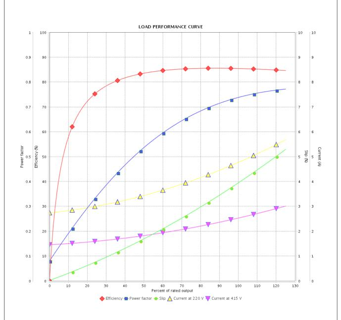
Performance : 220/415 V 50 Hz 6P Rated current : 4.73/2.51 A Moment of inertia (J) : 0.0118 kgm<sup>2</sup> **LRC** Duty cycle : Cont.(S1) : 6.3 Insulation class Rated torque : 1.13 kgfm : F Locked rotor torque : 220 % Service factor : 1.15 Breakdown torque : 290 % Temperature rise : 80 K Rated speed : 960 rpm Design : B
