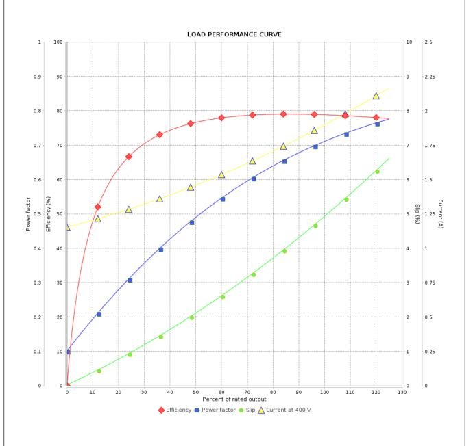
Performance : 400 V 50 Hz 6P IE2 : 1.94 A : 0.0067 kgm<sup>2</sup> Rated current Moment of inertia (J) **LRC** : 5.2 Duty cycle : Cont.(S1) : 0.764 kgfm Insulation class Rated torque : F Locked rotor torque : 229 % Service factor : 1.00 Breakdown torque : 260 % Temperature rise : 80 K Rated speed : 950 rpm Design : B Rev. Performed Checked Date **Changes Summary** Performed by Checked by Revision Page
