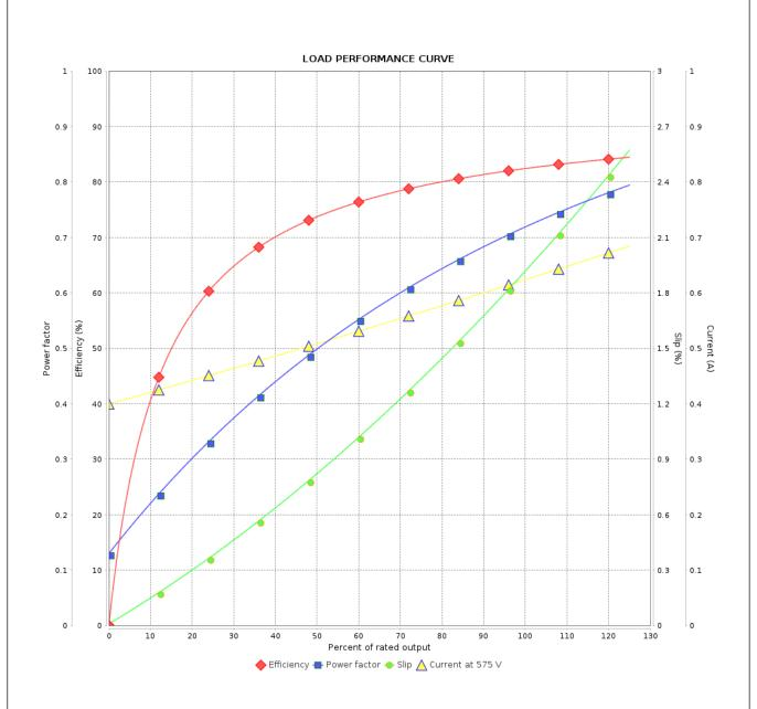
: 575 V 60 Hz 4P Performance : 0.625 A : 0.0046 kgm<sup>2</sup> Rated current Moment of inertia (J) **LRC** : 8.8 Duty cycle : Cont.(S1) : 0.206 kgfm Insulation class : F Rated torque Locked rotor torque : 280 % Service factor : 1.25 Breakdown torque : 400 % Temperature rise : 80 K Rated speed : 1765 rpm
