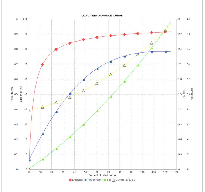
Performance : 575 V 60 Hz 8P : 15.7 A : 0.3448 kgm<sup>2</sup> Rated current Moment of inertia (J) **LRC** Duty cycle : Cont.(S1) : 5.5 Insulation class : 12.4 kgfm : F Rated torque Locked rotor torque : 200 % Service factor : 1.25 Breakdown torque : 229 % Temperature rise : 80 K Rated speed : 880 rpm Design : B Rev. Performed Checked Date **Changes Summary** Performed by
