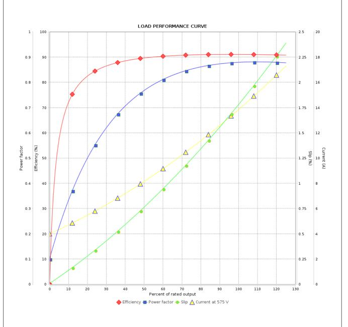
Performance : 575 V 60 Hz 2P : 13.8 A : 0.0530 kgm<sup>2</sup> Rated current Moment of inertia (J) **LRC** : 6.7 Duty cycle : Cont.(S1) Insulation class Rated torque : 3.08 kgfm : F Locked rotor torque : 220 % Service factor : 1.25 Breakdown torque : 270 % Temperature rise : 80 K Rated speed : 3532 rpm Design : B Rev. Performed Checked Date **Changes Summary** Performed by Checked by Revision Page
