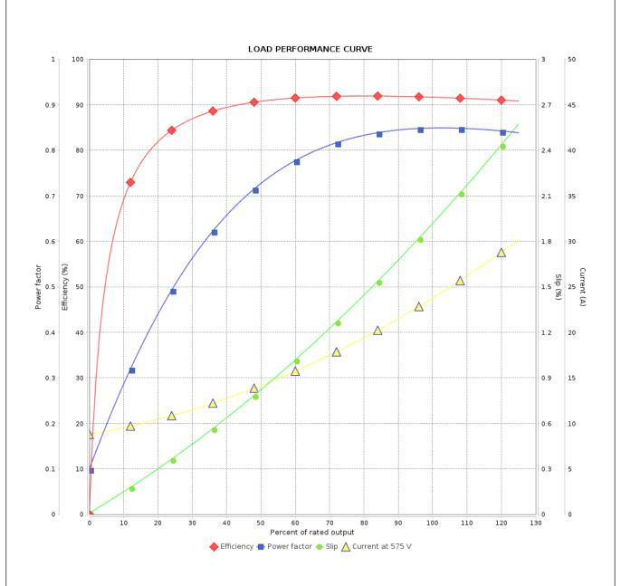
Performance : 575 V 60 Hz 2P : 0.0456 kgm<sup>2</sup> Rated current : 23.8 A Moment of inertia (J) **LRC** Duty cycle : Cont.(S1) : 6.5 Insulation class Rated torque : 5.14 kgfm : F Locked rotor torque : 200 % Service factor : 1.15 Breakdown torque : 260 % Temperature rise : 80 K Rated speed : 3530 rpm Design : B Rev. Performed Checked Date **Changes Summary** Performed by
