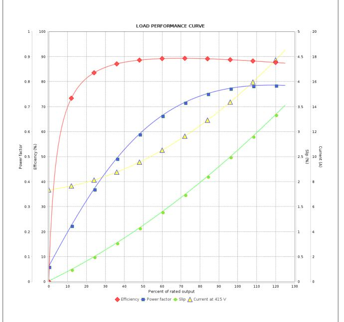
Performance : 415 V 50 Hz 8P IE3 : 15.1 A : 0.3034 kgm<sup>2</sup> Rated current Moment of inertia (J) **LRC** Duty cycle : Cont.(S1) : 5.2 : 9.94 kgfm Insulation class Rated torque : F Locked rotor torque : 190 % Service factor : 1.15 Breakdown torque : 229 % Temperature rise : 105 K Rated speed : 730 rpm Design : B Rev. Performed Checked Date **Changes Summary** Performed by
