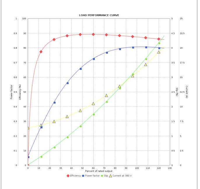
Performance : 380 V 50 Hz 8P IE3 : 16.1 A : 0.3034 kgm<sup>2</sup> Rated current Moment of inertia (J) **LRC** : 4.4 Duty cycle : Cont.(S1) Insulation class Rated torque : 10.0 kgfm : F Locked rotor torque : 150 % Service factor : 1.00 Breakdown torque : 190 % Temperature rise : 105 K Rated speed : 725 rpm Design : B Rev. Performed Checked Date **Changes Summary** Performed by
