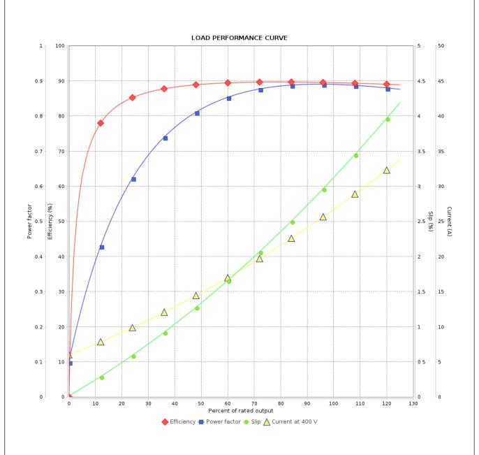
Performance : 400 V 50 Hz 2P IE1 : 0.0647 kgm<sup>2</sup> Rated current : 27.2 A Moment of inertia (J) **LRC** Duty cycle : Cont.(S1) : 5.7 : 5.00 kgfm Insulation class Rated torque : F Locked rotor torque : 180 % Service factor : 1.00 Breakdown torque : 210 % Temperature rise : 105 K Rated speed : 2905 rpm Design : B Rev. Performed Checked Date **Changes Summary** Performed by Checked by Revision Page
