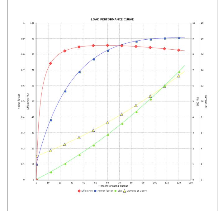
Performance : 380 V 50 Hz 2P : 11.1 A Rated current Moment of inertia (J) : 0.0069 kgm<sup>2</sup> **LRC** : 5.4 Duty cycle : Cont.(S1) : 1.92 kgfm : F Rated torque Insulation class Locked rotor torque : 150 % Service factor : 1.00 Breakdown torque : 210 % Temperature rise : 105 K Rated speed : 2835 rpm Design : B
