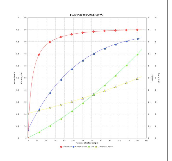
: 690 V 60 Hz 4P Performance : 4.38 A Rated current Moment of inertia (J) : 0.0156 kgm<sup>2</sup> **LRC** : 7.1 Duty cycle : Cont.(S1) : 2.07 kgfm Insulation class : F Rated torque Locked rotor torque : 229 % Service factor : 1.15 Breakdown torque : 300 % Temperature rise : 80 K Rated speed · 1750 rpm ·R Design
