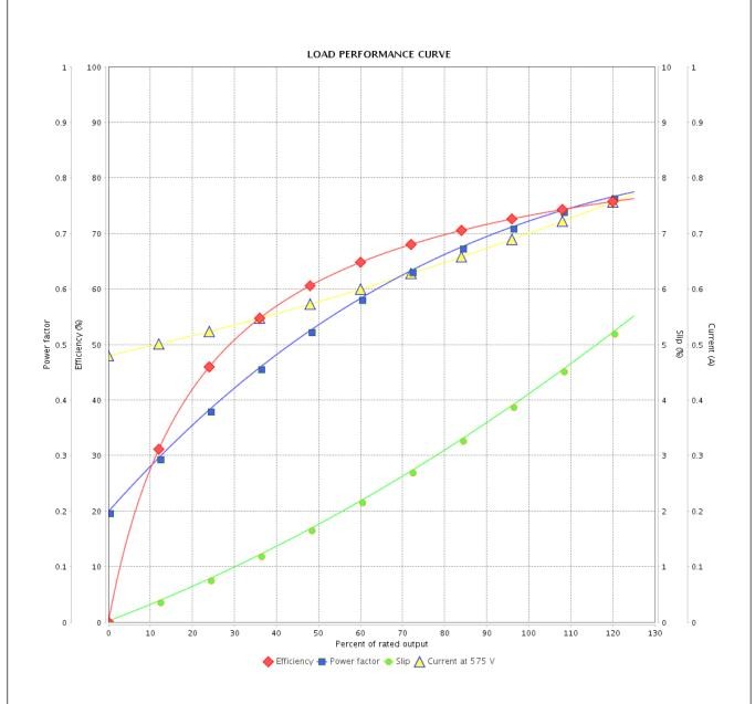
Performance : 575 V 60 Hz 2P : 0.0006 kgm<sup>2</sup> Rated current : 0.703 A Moment of inertia (J) **LRC** Duty cycle : Cont.(S1) : 7.3 : 0.105 kgfm Insulation class : F Rated torque Locked rotor torque : 370 % Service factor : 1.60 Breakdown torque : 400 % Temperature rise : 80 K Rated speed : 3450 rpm
