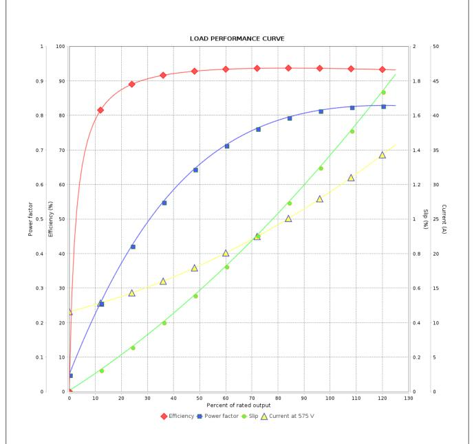
Performance : 575 V 60 Hz 4P : 28.8 A Rated current Moment of inertia (J) : 0.2175 kgm<sup>2</sup> **LRC** : 7.9 Duty cycle : Cont.(S1) Insulation class Rated torque : 12.3 kgfm : F Locked rotor torque : 290 % Service factor : 1.25 Breakdown torque : 320 % Temperature rise : 80 K Rated speed : 1775 rpm Design : B
