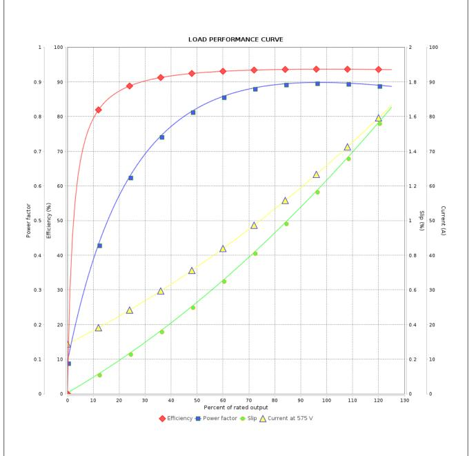
Performance : 575 V 60 Hz 2P : 0.5023 kgm<sup>2</sup> Rated current : 65.5 A Moment of inertia (J) **LRC** : 6.7 Duty cycle : Cont.(S1) : 15.3 kgfm Insulation class Rated torque : F Locked rotor torque : 200 % Service factor : 1.25 Breakdown torque : 250 % Temperature rise : 80 K Rated speed : 3555 rpm Design : B Rev. Performed Checked Date **Changes Summary** Performed by Checked by Revision Page
