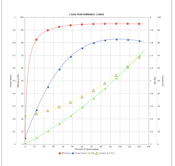
Performance : 575 V 60 Hz 4P : 0.9448 kgm<sup>2</sup> Rated current : 57.3 A Moment of inertia (J) **LRC** : 6.2 Duty cycle : Cont.(S1) Insulation class Rated torque : 24.5 kgfm : F Locked rotor torque : 220 % Service factor : 1.25 Breakdown torque : 240 % Temperature rise : 80 K Rated speed : 1780 rpm Design : B Rev. Performed Checked Date **Changes Summary** Performed by Checked by Revision Page
