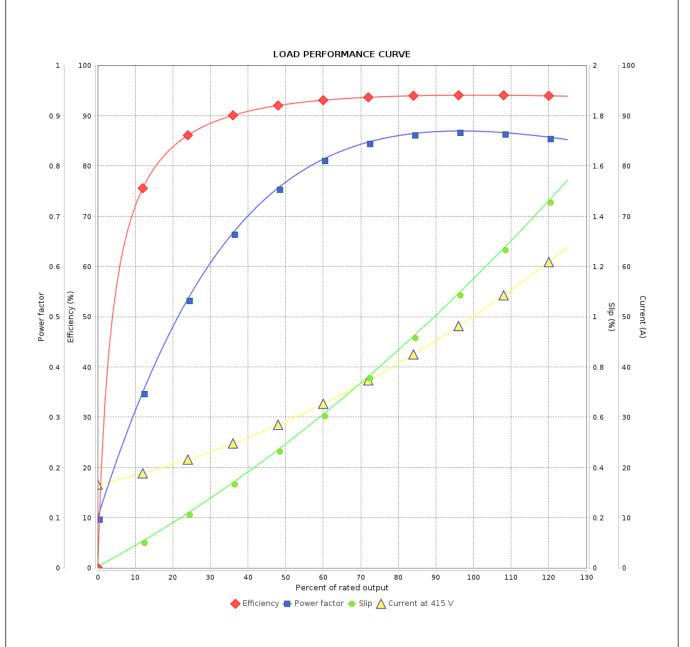
Performance : 415 V 50 Hz 2P IE3 : 0.2284 kgm<sup>2</sup> Rated current : 51.0 A Moment of inertia (J) **LRC** : 7.9 Duty cycle : Cont.(S1) : 9.79 kgfm Insulation class Rated torque : F Locked rotor torque : 280 % Service factor : 1.00 Breakdown torque : 300 % Temperature rise : 80 K Rated speed : 2965 rpm Design : B Rev. Performed Checked Date **Changes Summary** Performed by
