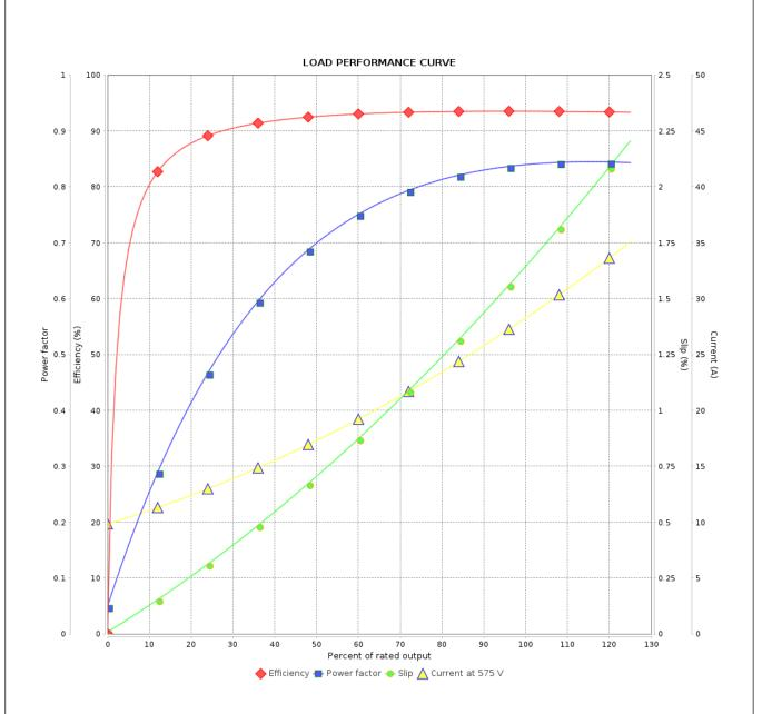
Performance : 575 V 60 Hz 4P : 0.2467 kgm<sup>2</sup> Rated current : 28.1 A Moment of inertia (J) **LRC** Duty cycle : Cont.(S1) : 6.1 Insulation class Rated torque : 12.3 kgfm : F Locked rotor torque : 240 % Service factor : 1.25 Breakdown torque : 240 % Temperature rise : 80 K Rated speed : 1770 rpm Design : B Rev. Performed Checked Date **Changes Summary** Performed by
