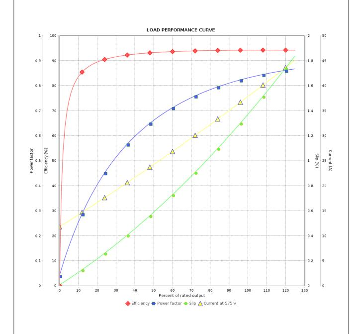
Performance : 575 V 60 Hz 4P Rated current : 38.6 A Moment of inertia (J) : 0.3441 kgm<sup>2</sup> **LRC** : 7.7 Duty cycle : Cont.(S1) : 16.4 kgfm : F Rated torque Insulation class Locked rotor torque : 270 % Service factor : 1.15 Breakdown torque : 300 % Temperature rise : 80 K Rated speed : 1780 rpm Design : B
