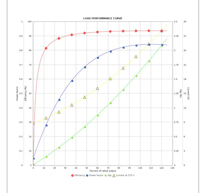
: 575 V 60 Hz 4P Performance : 23.6 A Rated current Moment of inertia (J) : 0.1914 kgm<sup>2</sup> **LRC** : 6.2 Duty cycle : Cont.(S1) : 10.3 kgfm Insulation class : F Rated torque Locked rotor torque : 240 % Service factor : 1.15 Breakdown torque : 270 % Temperature rise : 105 K Rated speed · 1770 rpm Design
