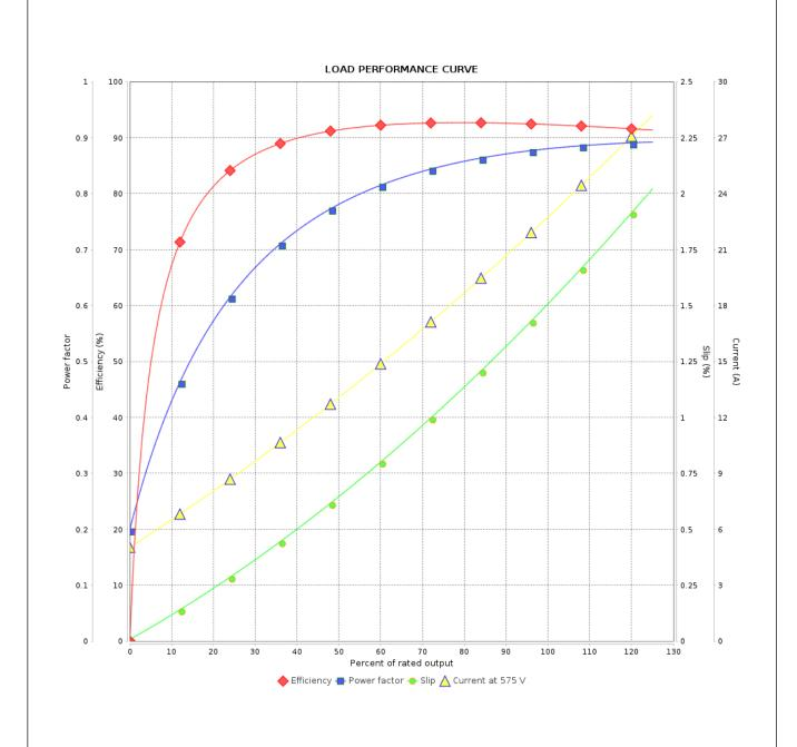
Performance : 575 V 60 Hz 2P : 22.8 A Rated current Moment of inertia (J) : 0.1086 kgm<sup>2</sup> **LRC** : 6.7 Duty cycle : Cont.(S1) : 5.12 kgfm Insulation class : F Rated torque Locked rotor torque : 240 % Service factor : 1.15 Breakdown torque : 240 % Temperature rise : 80 K Rated speed : 3545 rpm Design : B
