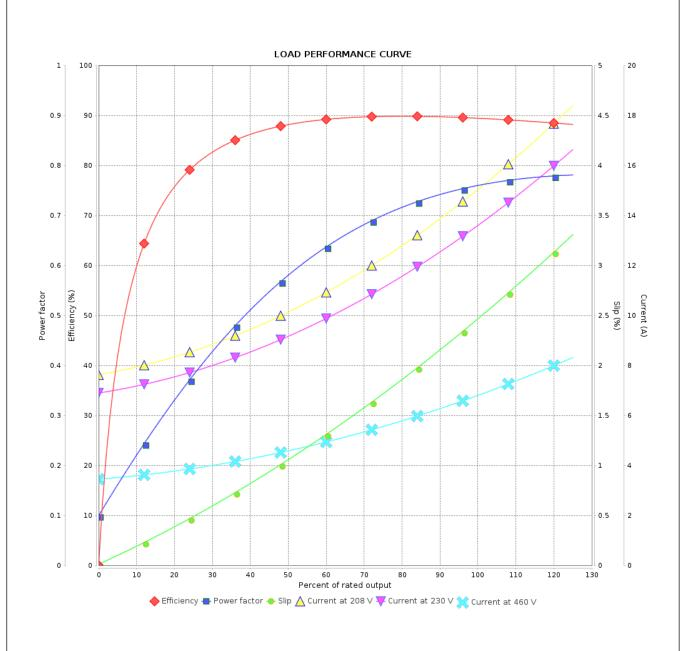
Performance : 230/460 V 60 Hz 6P : 13.7/6.83 A : 0.0620 kgm<sup>2</sup> Moment of inertia (J) Rated current **LRC** Duty cycle : Cont.(S1) : 6.8 Insulation class : 3.10 kgfm : F Rated torque Locked rotor torque : 170 % Service factor : 1.15 Breakdown torque : 260 % Temperature rise : 80 K Rated speed : 1170 rpm Design : B Rev. Performed Checked Date **Changes Summary** Performed by Checked by Revision Page
