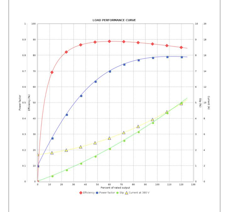
Performance : 380 V 50 Hz 6P IE3 : 8.20 A Rated current Moment of inertia (J) : 0.0620 kgm<sup>2</sup> **LRC** : 5.5 Duty cycle : Cont.(S1) : 3.78 kgfm Insulation class : F Rated torque Locked rotor torque : 150 % Service factor : 1.00 Breakdown torque : 215 % Temperature rise : 80 K Rated speed · 060 rpm Design
