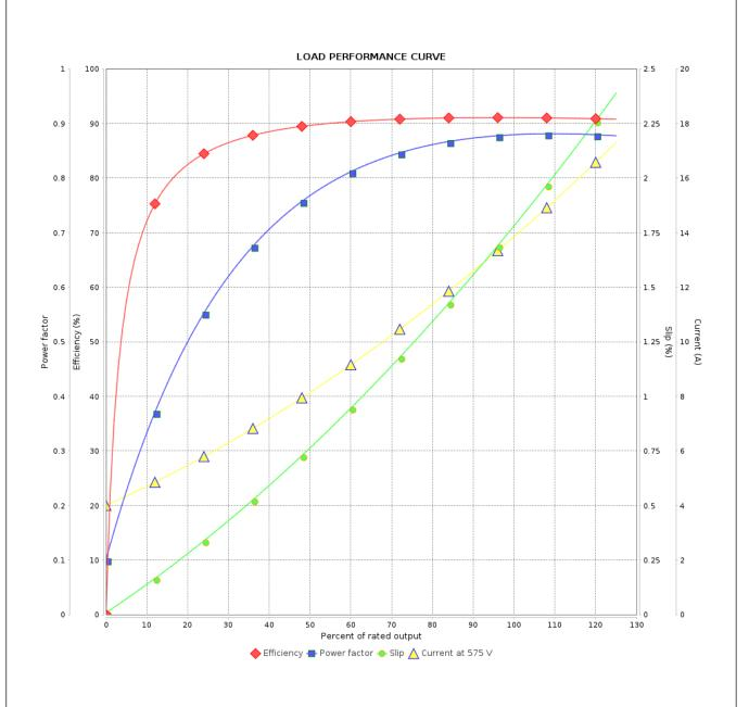
Performance : 575 V 60 Hz 2P : 13.8 A : 0.0530 kgm<sup>2</sup> Rated current Moment of inertia (J) **LRC** : 6.7 Duty cycle : Cont.(S1) Insulation class Rated torque : 3.08 kgfm : F Locked rotor torque : 200 % Service factor : 1.25 Breakdown torque : 260 % Temperature rise : 80 K Rated speed : 3535 rpm Design : B Rev. Performed Checked Date **Changes Summary** Performed by Checked by Revision Page
