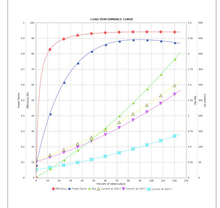
Performance : 230/460 V 60 Hz 2P : 224/112 A Rated current Moment of inertia (J) : 0.5561 kgm<sup>2</sup> **LRC** : 6.5 Duty cycle : Cont.(S1) : F Rated torque : 20.5 kgfm Insulation class Locked rotor torque : 240 % Service factor : 1.25 Breakdown torque : 260 % Temperature rise : 80 K Rated speed : 3545 rpm Design : B
