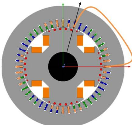
Figure 3: Fractional pitch winding (5/6)
