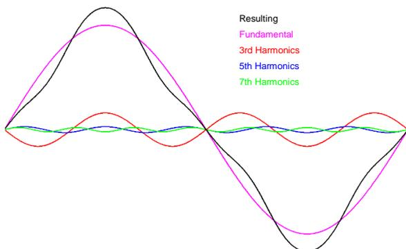
Figure 1: Relation between waveform and harmonics
