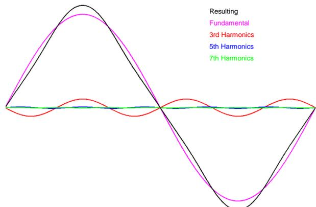
Figure 6: Harmonics with 5/6 pitch winding
