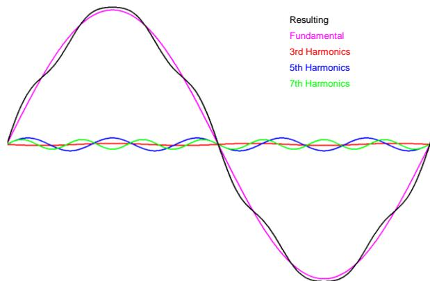
Figure 5: Harmonics with 2/3 pitch winding
