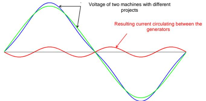
Figure 8: Circulating neutral current and voltages resulting from the two machines
