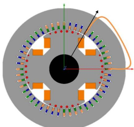
Figure 4: Fractional pitch winding (2/3)
