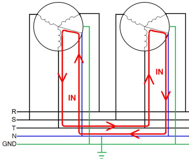
Figure 7: Circulating neutral current
