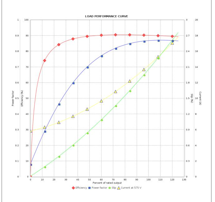
Performance : 575 V 60 Hz 2P : 14.1 A : 0.0232 kgm<sup>2</sup> Rated current Moment of inertia (J) **LRC** Duty cycle : Cont.(S1) : 6.8 Insulation class Rated torque : 3.09 kgfm : F Locked rotor torque : 229 % Service factor : 1.15 Breakdown torque : 280 % Temperature rise : 80 K Rated speed : 3525 rpm Design : B Rev. Changes Summary Checked Performed Date
