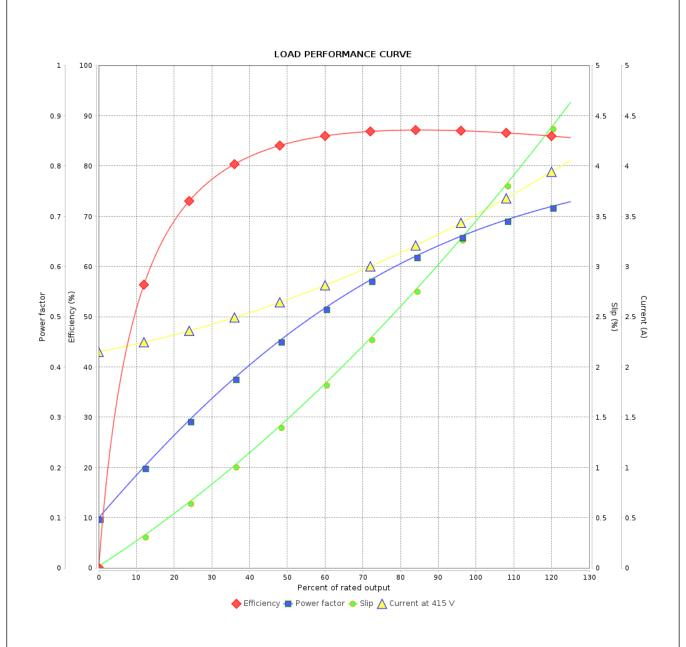
Performance : 415 V 50 Hz 6P IE4 : 0.0262 kgm<sup>2</sup> Rated current : 3.58 A Moment of inertia (J) **LRC** : 7.1 Duty cycle : Cont.(S1) : 1.50 kgfm Insulation class Rated torque : F Locked rotor torque : 310 % Service factor : 1.00 Breakdown torque : 330 % Temperature rise : 80 K Rated speed : 965 rpm Design : B Rev. Performed Checked Date **Changes Summary** Performed by
